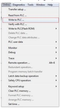
10、在弹出的对话框中,对需下载的 PLC 程序进行设置,如下图所示 In the prompted dialog box, set PLC program which is needed to download, as below image:
