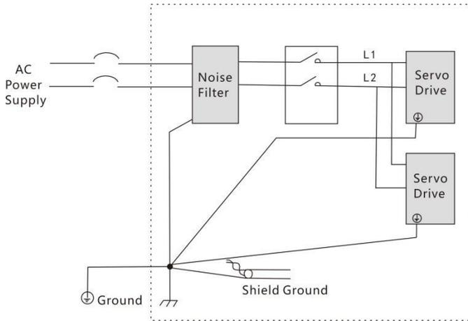
Pic 4.16 Ground Connection Handling Of Noise Filter
