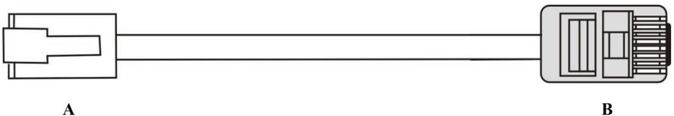
Pic 4.10 Parallel Cable Diagram Of Multi Drives
