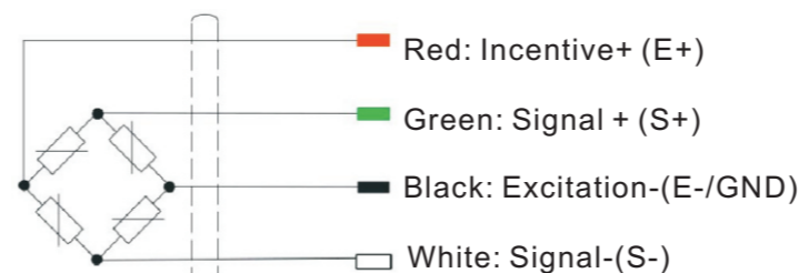
Diagram 14 Load cell sensor wiring
